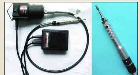
Fig 5. The Dremel heavy-duty flex shaft tool has a 12.7-mm handpiece and a foot control speed lever.
