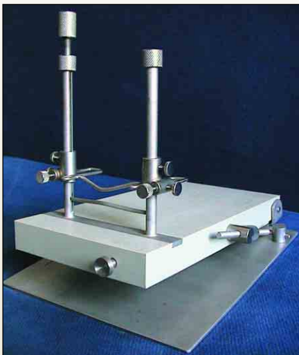
Fig 1. The rodent table retractor/restrainer (also called "tabletop rodent gag") is a special platform for restraining anesthetized rabbits and rodents with the mouth held open and the cheeks retracted. Using this device, an assistant does not need to hold the retraction
